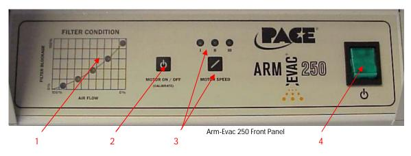
The Arm-Evac 250 has a graphical Filter Condition Display (1) which continuously monitors filter condition. As the system filter(s) collect particulates, LED's on the Filter Condition Display will illuminate along the graphical curve of the display.
